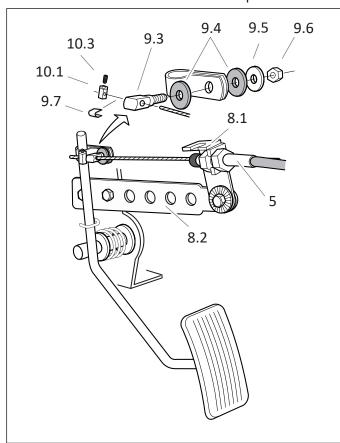
If throttle pedal have an idle contact, kick-down switch or electronic cruise control is not suitable, the servo cable should be mounted directly to the pedal.
