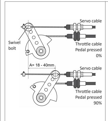
Find a connection point in the throttle mechanism where the cruise control cable stroke A is between 18 and 40 mm when throttle pedal is pressed from 0 to about 90%. Throttle cable stroke must always be longer than stroke of servo cable!
