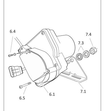
Fasten servo cover 6.1 it using the bolt with spring washer 6.4 and screw 6.5.
