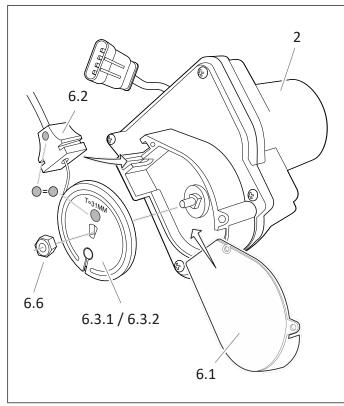
Place the pulley 6.3.1 or 6.3.2 on the axle of the electronic servo 2, with the correct stroke size visible on the outside, secure it with the M6 lock nut 6.6. Install the cruise control cable with triangular plastic block 6.2 to the servo so, that the visible colour on it matches the colour on the pulley.
