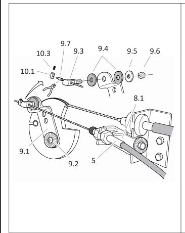
Determine the most suitable throttle linkage. Mount cable bracket 8.1. It can be used as one piece or with extension 8.2 or bent and trimmed in numerous ways.
