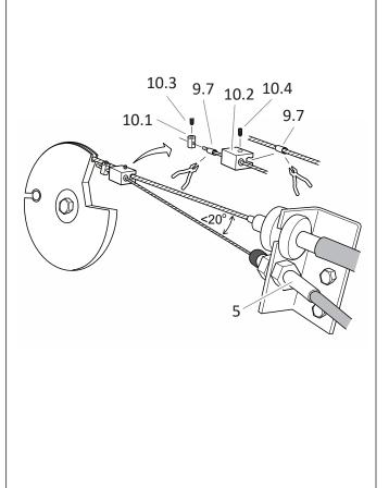
Determine the most suitable throttle linkage so that the angle between servo and throttle cable is less than 20<sup>o</sup>. Mount cable bracket 8.1 like described on ch. 3.1 or find an attachment point where bracket is not needed.
