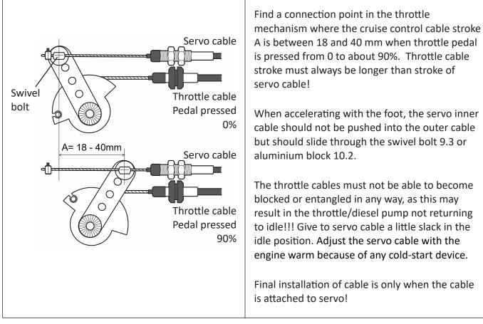
3.2 Servo cable attachment to the throttle pulley
