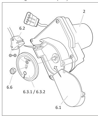
Place the pulley 6.3.1 or 6.3.2 on the axle of the electronic servo 2, with the written correct stroke size visible on the outside, secure it with the M6 lock nut 6.6. Install the cruise control cable with triangular plastic block 6.2 to the servo so, that the visible colour on it matches the colour on the pulley.
