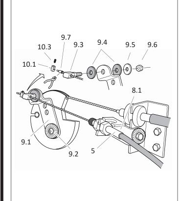
Determine the most suitable throttle linkage. Mount cable bracket 8.1. It can be used as one piece or with extension 8.2 or bent and trimmed in numerous ways.
