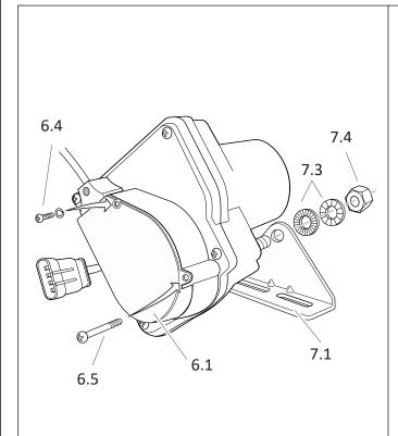
Fasten servo cover 6.1 it using the bolt with spring washer 6.4 and screw 6.5.
