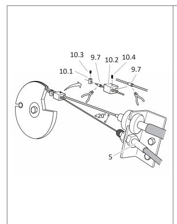
Determine the most suitable throttle linkage so that the angle between servo and throttle cable is less than 20°. Mount cable bracket 8.1 like described on ch. 3.1 or find an attachment point where bracket is not needed.
