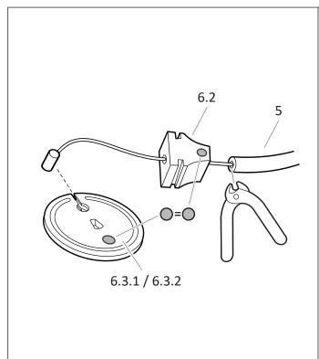
Use a caliper to determine the cruise control cable stroke A described in ch. 3.1. Based on this length, the choice of pulley to be used is made. Ideally, the stroke of the chosen pulley should be a few millimetres shorter than distance A.
