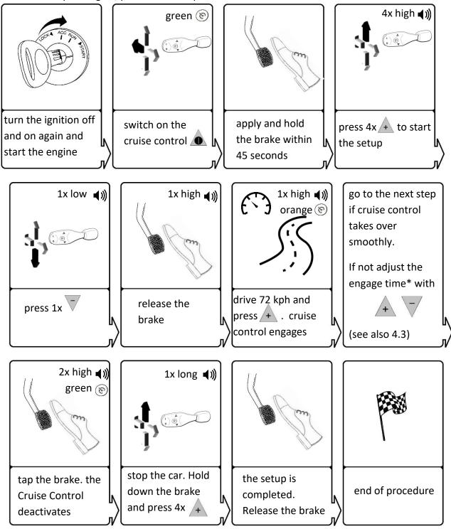
\* During speed calibration, the reaction time of switching on the Cruise Control can be adjusted directly. The reaction time is properly adjusted if the Cruise Control keeps the speed exactly constant when engaged.
