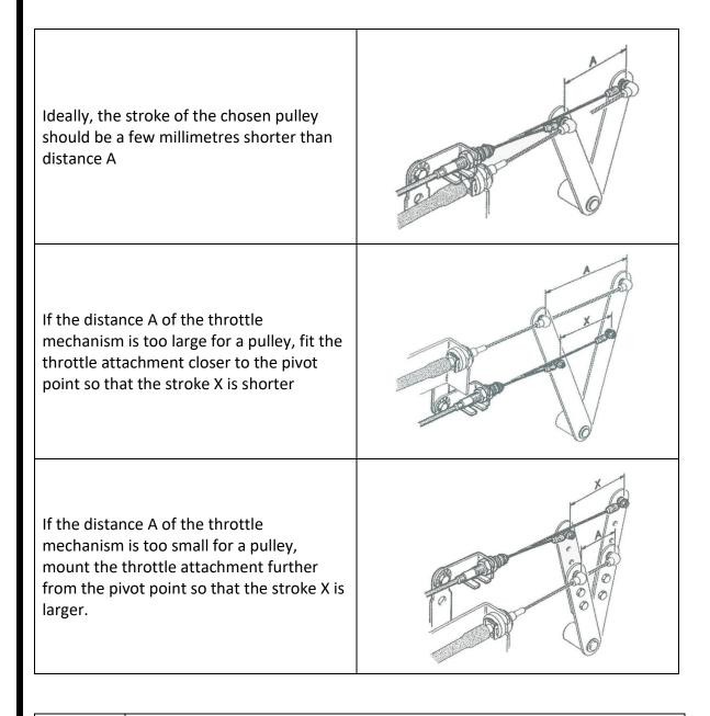
Always check the smooth operation of the throttle, throttle cable and servo cable by operating the throttle mechanism with your foot and hand. These should not be able to block in any way.
